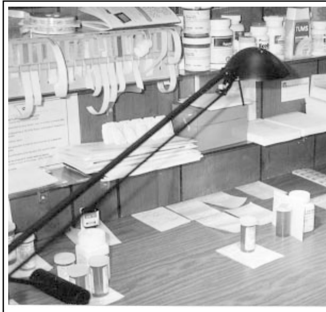
Prototype 8: High-Intensity Task Light / Produced a visual boost to aid discrimination of difficult to read information on scripts & labels.
